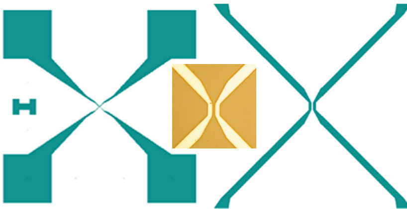
Figure 3.9: Lithography mask design with Clewin® 3.0 software. The optical microscope image in the middle shows a 2 \mu\text{m} gap between the electrodes.
