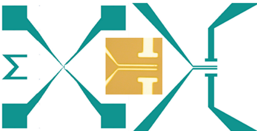
Figure 3.10: Lithography mask design with Clewin® 3.0 software. The optical microscope image in the middle shows a 2 \mu\text{m} gap between the electrodes.
